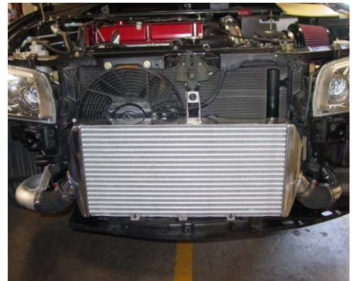
We offer 23 1/2" x 113/4" x 3 3/8" intercoolers will fit the stock piping and elbows or Injens intake system. Intercooler cores are made in the USA.
