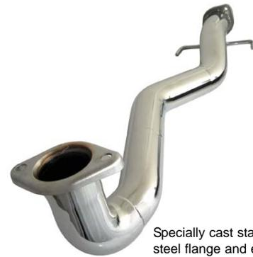
Specially cast stainless steel flange and elbow.
