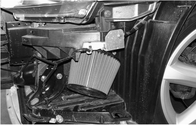
Press the 3 1/2" filter over the end of the secondary intake and tighten the clamp on the filter neck.
