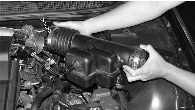
Loosen clamp at the throttle body and remove the air intake duct. **At this point, it will be necessary to remove the front bumper. Remove 9 clips on top of the bumper, two 10mm screws on each side of the bumper, four additional sheet screws and 5 plastic clips.**
