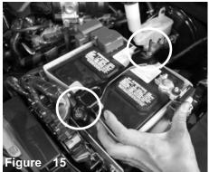
Loosen the 2 10mm nuts holding in the battery bracket tie down.
