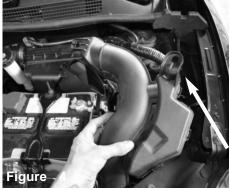
Lift up and remove the factory intake snorkel plastic piece.
