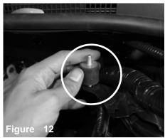
Install the M6 vibramount to the thredded insert from step 5.
