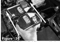
Now push the battery to the left/passenger side closer to the engine. This will give more clearance from the tube touching battery.Note: Injen Technology is not responsible or liable for damage to battery or intake system and will not be covered under warranty for inproper installation or clearance issues.
