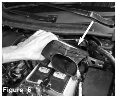
Now lift up and remove the lower part of the air box out of the vehicle.
