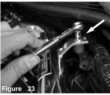
Tighten the vibra mount using 10mm socket and ratchet.
