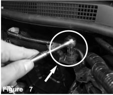
Loosen the 10mm bolt holding in the upper part of the air box. Remove the bolt from the
