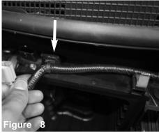
Remove the MAF sensor line away from the upper part of the airbox.
