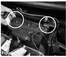
Now, un-clip the factory clips holding in the lower part of the intake air box.
