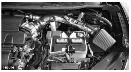
Congratulations! You have just completed the installation of this intake system. Periodically, check the alignment of the intake, normal wear and tear can cause nuts and bolts to come loose. <u>Note: Check clearance and adjust if needed! Failure to check the alignment and adjust the intake can cause damage that will void the warranty. Injen Technology is not responsible for any damages caused by/from improper installation.</u>
