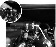
A) Install the hose with clamps provided to the crank case hard line.B) Tighen the clamp on the hard line only.
