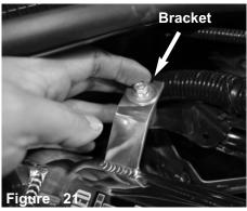
Now secure the bracket using provided fender washer and M6 nut.
