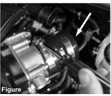
Install the hump hose with clamps provided to the throttle body and tighten clamp on throttle body.
