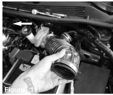
Now pull the hard crank case line from the intake tube. Remove the intake tube from the vehicle.
