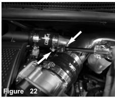
Tighten the clamp on the throttle body.
