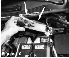
Lift up and remove the upper part of the air box.
