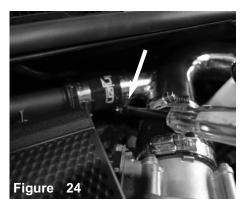
Secure the hard crank case line and tighten using 8mm nut driver.
