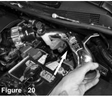
Install the intake tube into vehicle and position to the hump hose and the bracket to the vibramount.
