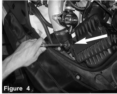
With 10mm socket and ratchet, loosen the bolt holding in the air box.
