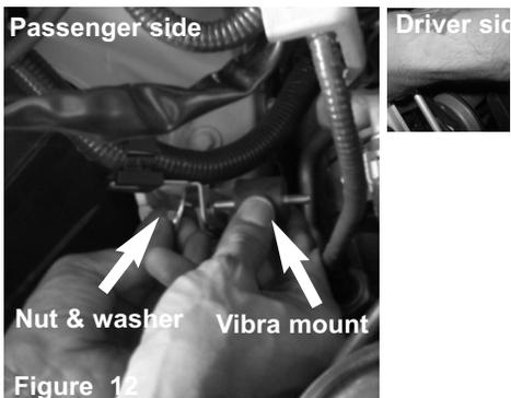
Install the vibra mounts to the brackets and secure. See above images for passenger and driver side.
