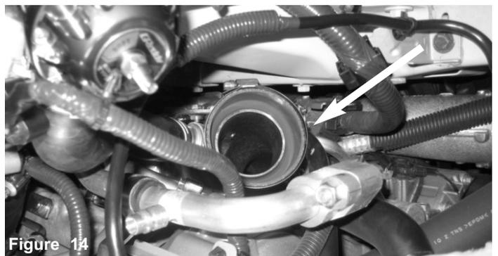
On both sides of the vehicle, install the step hose to turbo with the clamps provided. Position the clamps allowing for easier access. Tighten the clamp on the turbo only.
