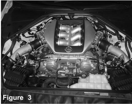
Complete stock intake system, Disconnect battery. Remove both sides of stock intakes. Passenger side shown, both are exactly the same when removing.
