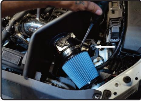
25. Install the air filter to the intake tube and secure using 8mm nut driver.
