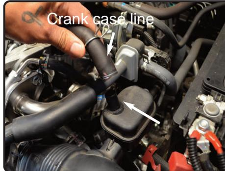
3. Push the factory clamp in and pull back the crank case line away from the intake tube.
