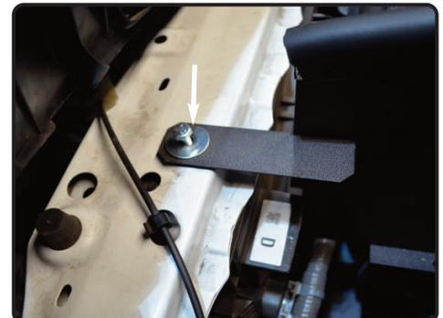
**16.** Place tab over the threaded insert. Secure using provided M6 hex screw and fender washer.
