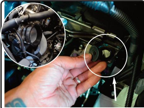
**13.** Remove the 1 grommet from the oem air box mounting brackets. Install the urethane step hose with clamps provided to the throttle body.
