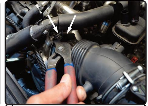
4. With pliers or channel locks carefully de-press the large clamp on the throttle body. Pull back the intake tube from the throttle body.
