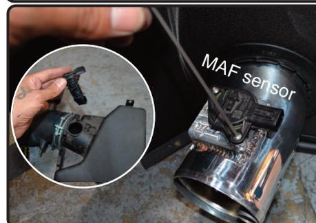
11. Remove the MAF sensor using phillips screwdriver. Install into the new intake tube and secure using provided M4 button head screws.
