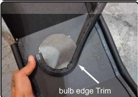
9. Partially install the bulb edge trim to the hole inside the heatshield.
