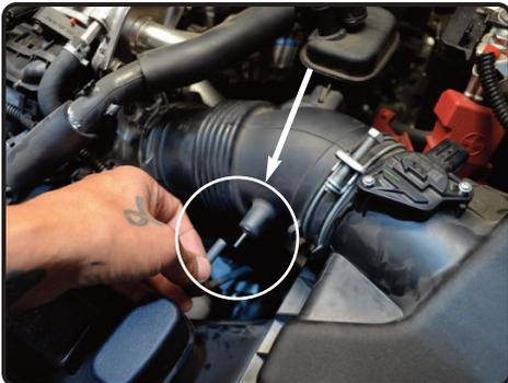
5. Pull back the vacuum line away from the intake tube.
