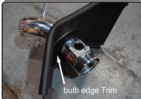
10. Install the intake tube through the hole with MAF sensor pad side. Maneuver and finish the rest of the bulb edge trim installation.
