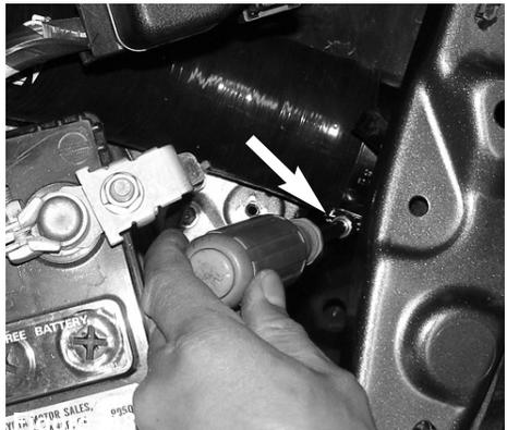
The silicone hose clamp is now tightened as shown above.
