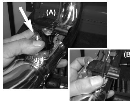
A) Install the MAF sensor into the intake tube. B) Secure using provided M4 screws and tighten.
