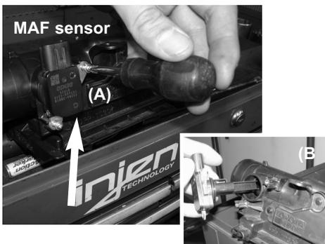
A) Loosen the 2 screws holding in the MAF sensor using phillips screwdriver. B) Remove the MAF sensor from the air box.
