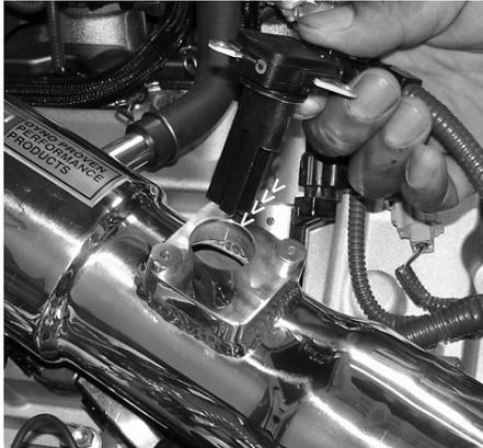
Prior to inserting the MAFS into the machined adapter, use a light weight oil around the O-ring then press the MAFS sensor into the open hole.
