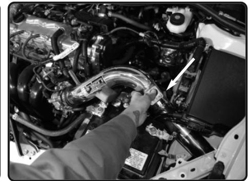
**15.** Now rotate and position the tube to the hose and the bracket to the vibramount.
