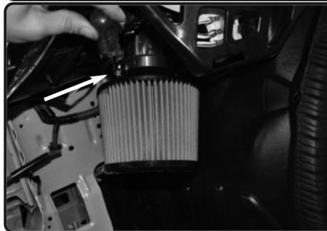
**22.** Install the air filter to the intake tube. Secure and tighten using 8mm nut driver.
