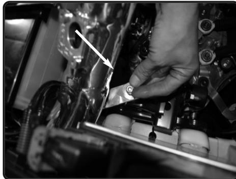
**17.** Secure the bracket using provided m6 nut and washer.
