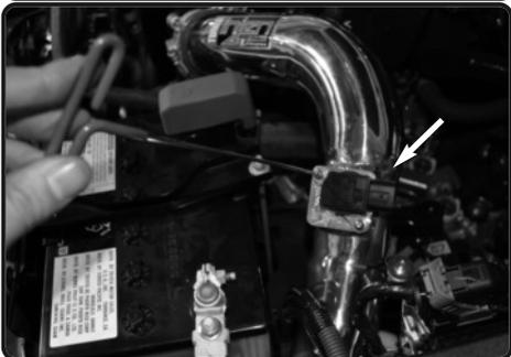
**20.** Re-install the MAF sensor into the new injen intake tube. Secure and tighten using M4 screws provided and tighten using 2.5mm allen key.
