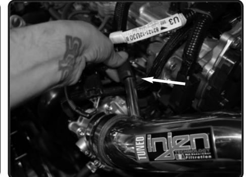
**19.** Re-connect the crank-case line to the fitting on the injen intake tube.
