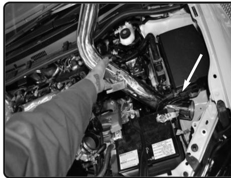
**14.** Install the intake tube through the battery cable tunnel.
