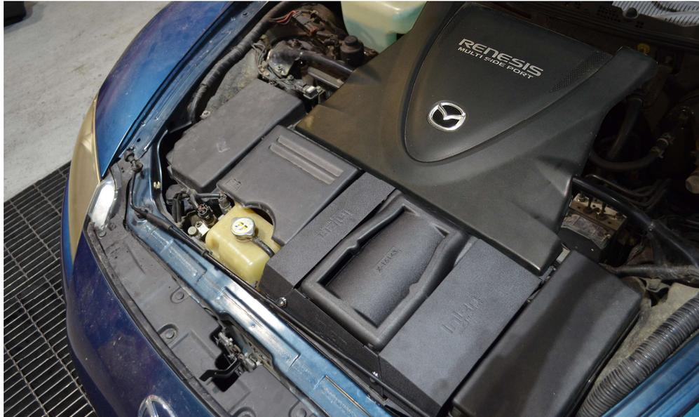
Align the entire intake for best possible fit. Once you have aligned and made sure that the length of the intake is free from any moving parts, continue to tighten all nuts, bolts and clamps. Congratulations! You have just completed the installation of this intake system. Periodically, check the alignment of the intake, normal wear and tear can cause nuts and bolts to come loose. Failure to check the alignment and adjust the intake can cause damage that will void the warranty.
