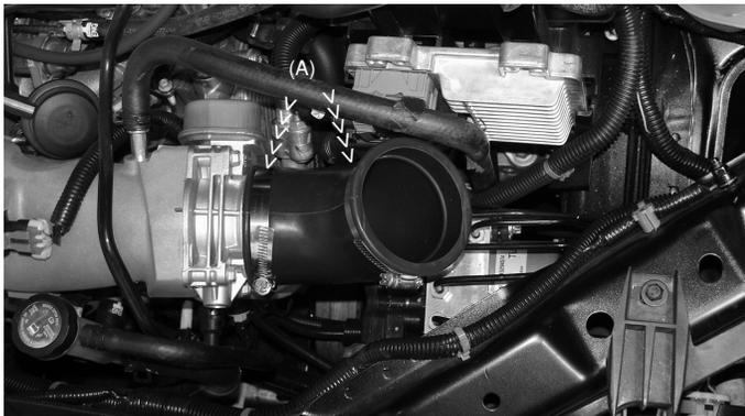
Prior to installing the elbow place a clamp over each end of the elbow (A). Take the 60 degree elbow and press the 2 7/8" over the throttle body. Position the 3" inlet side so that it faces upward.
