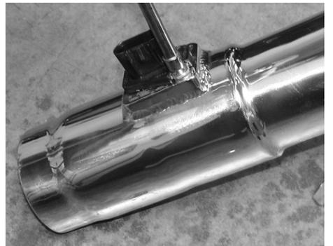
Close up of MR Technology at its best. Once the mass air sensor is inserted into the adapter, use the 4mm button head screws to firmly secure the sensor in place.
