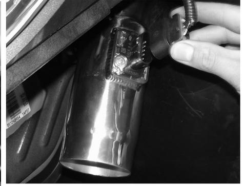
Once the intake has been carefully aligned, take the ECU harness and press it over the mass air sensor. You will hear a short snap when the harness has been properly connected.
