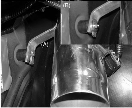
Once the top end has been pressed into the elbow continue to align the intake bracket to the vibr-mount stud(A). Use the 6mm nut and fender washer to fasten the intake in place (B).
