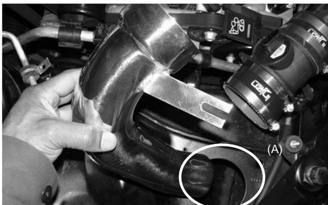
Installation of the cold air intake- Prior to installing the secondary intake press the vinyl trim around the inside diameter of the resonator opening (A). Once the vinyl trim is in place, lower the secondary intake into the resonator opening.
