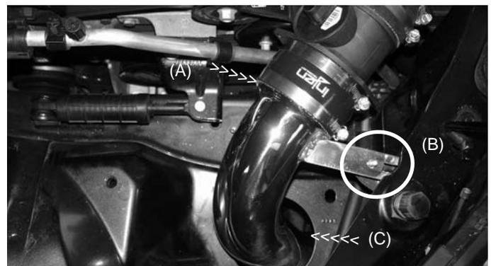
Press the large end of the intake into the 3 3/8" hose located on the mass air sensor (A). Align the intake bracket to the vibra-mount stud (B). Keep proper clearance around the resonator opening. The intake should not touch any area along the edge of the resonator opening (C).
