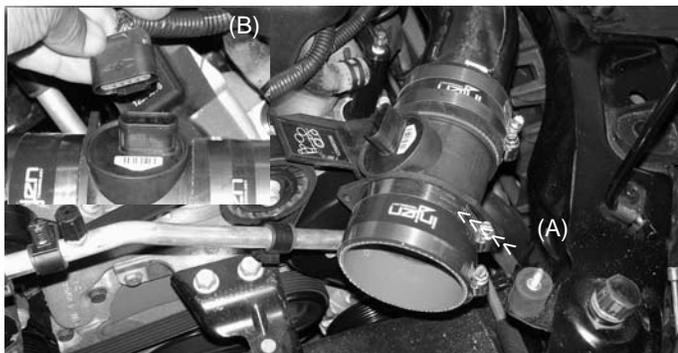
Take the 3 3/8" straight hose (injen logo) and press it over the inlet end of the mass air flow sensor (A). Take two medium clamps and place them on the end of the 3 3/8" hose, tighten the clamp on the mass air flow sensor side (A). Locate the male harness connector and press it over the female connecting point (B).
