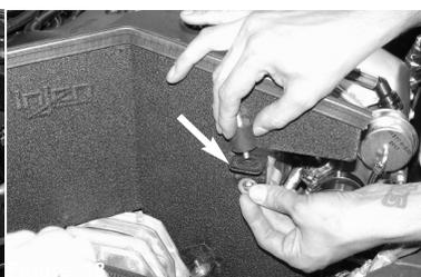
Place the male/male vibramount onto the bracket located on top of the lower heat shield bracket. Use a M6 nut to secure the vibramount to the bracket and then tighten the M6 nut with a 10mm ratchet.
