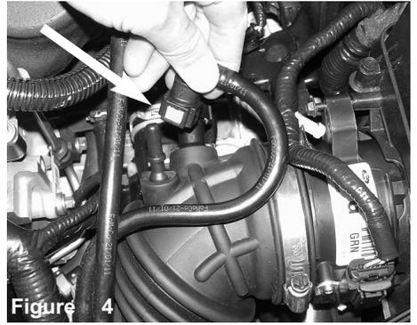
Figure 4 Disconnect the vacuum line from stock intake.
