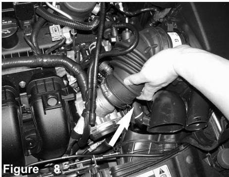
Figure 8 Pull back intake tube from throttle body.
