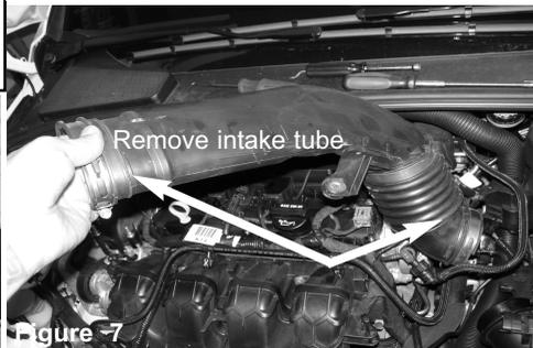
Figure 7 Carefully lift up and remove the stock intake tube from the vehicle.
