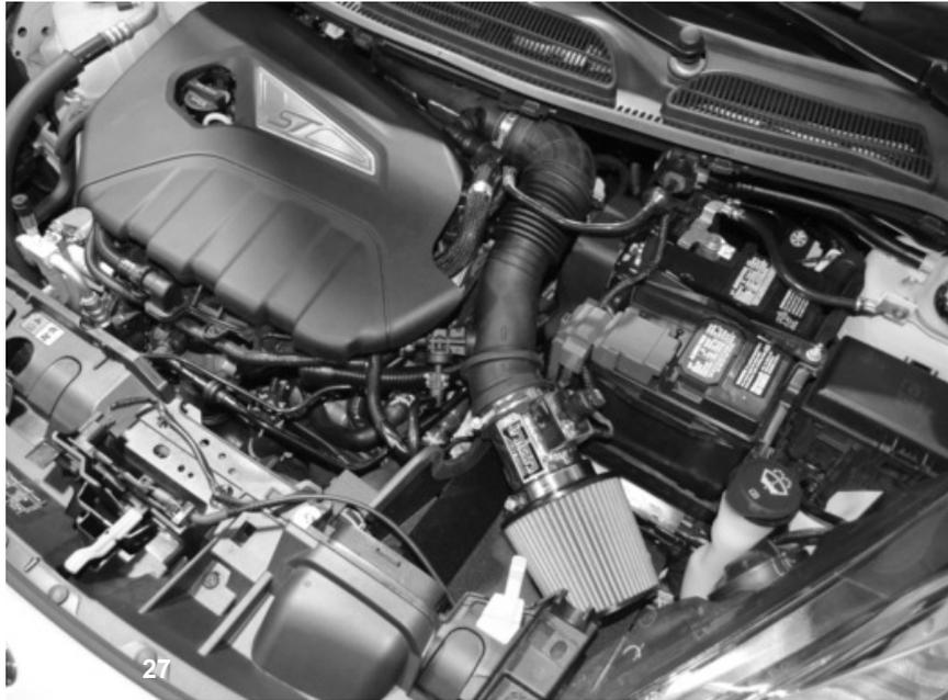
Congratulations! You have just completed the installation of this intake system. Periodically, check the alignment of the intake, normal wear and tear can cause nuts and bolts to come loose. **Note: Check clearance and adjust if needed! Failure to check the alignment and adjust the intake can cause damage that will void the warranty. Injen Technology is not responsible for any damages caused by/from improper installation.**
