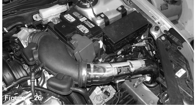
Congratulations! You have just completed the installation of this intake system. Periodically, check the alignment of the intake, normal wear and tear can cause nuts and bolts to come loose. **Note: Check clearance and adjust if needed! Failure to check the alignment and adjust the intake can cause damage that will void the warranty. Injen Technology is not responsible for any damages caused by/from improper installation.**
