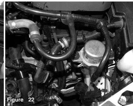
Re-install the vacuum assembly back into vehicle. Make sure everything is connected.
