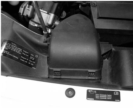
With 8mm socket and ratchet, loosen the 2 bolts holding in the factory scoop.
