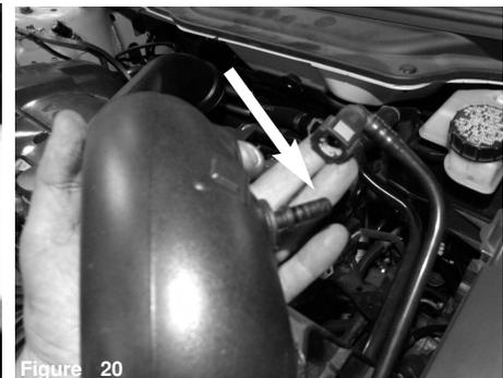
Disconnect the crank case port from the stock intake tube.
