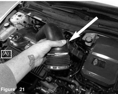
Remove the stock intake tube from vehicle.
