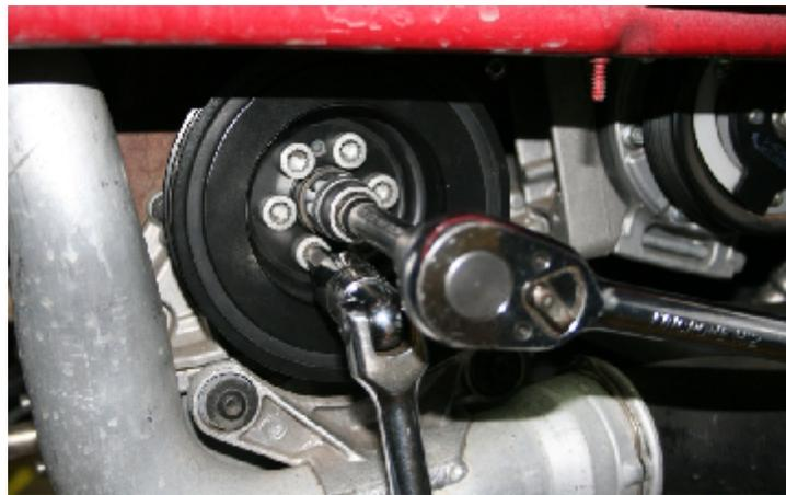
On 2006-2007.5 models the crank pulley bolts are 6mm hex socket heads and are stretch-type bolts. Make sure to use a good quality 6mm hex key, one that has no wear on the points or you may round the bolt sockets. Take care when undoing these bolts, as they can be quite tight and can be easy to round. If the bolt shows signs of starting to round before you can loosen it, try a product that freezes the bolt to help loosen it.
