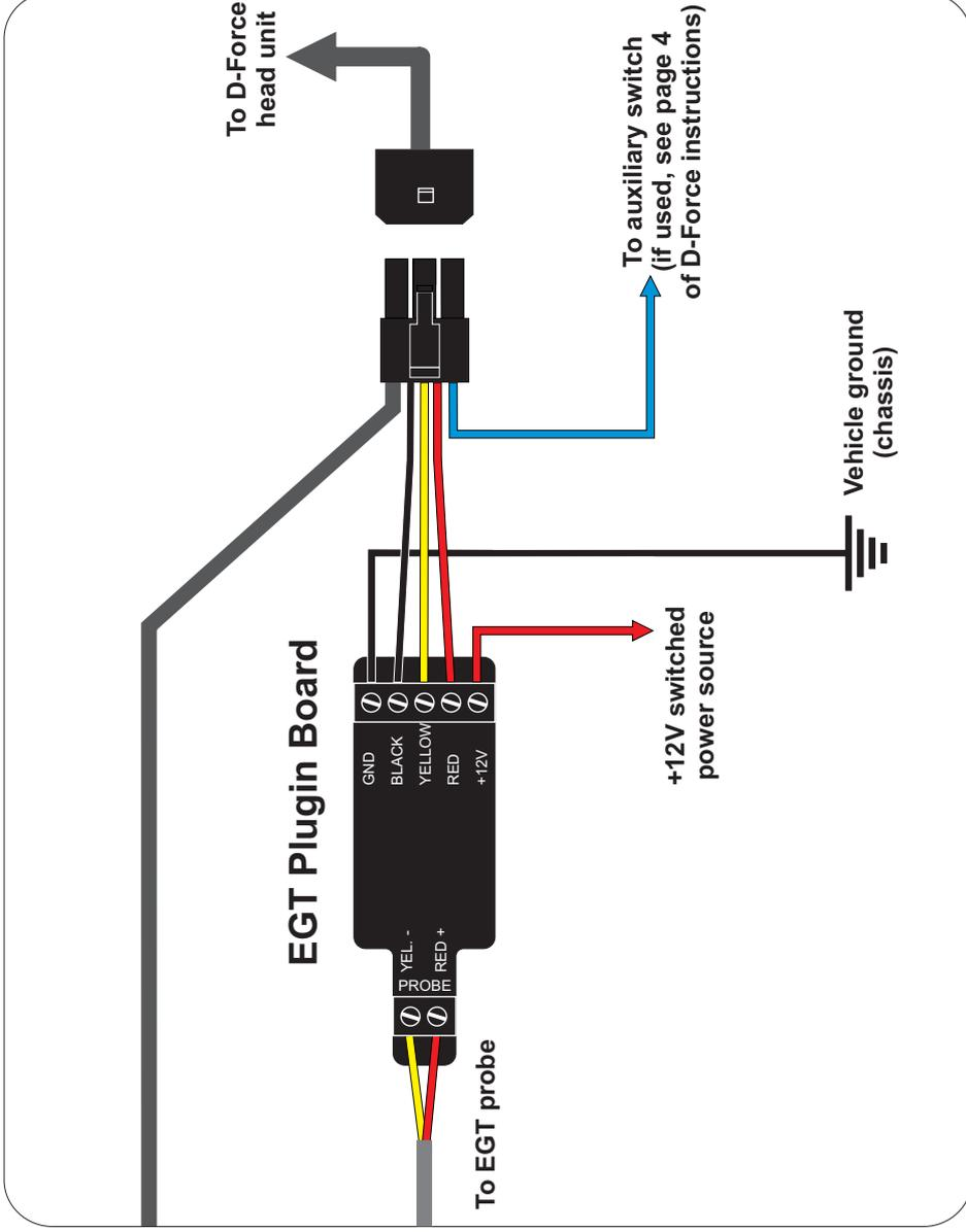
The EGT Plug-in board is designed to connect inline with the existing D-Force wiring loom via screw terminals. Take careful note of the wiring diagram above and double-check all connections before powering the unit up.
