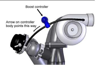
The third configuration is a typical installation for electronic boost controllers.
