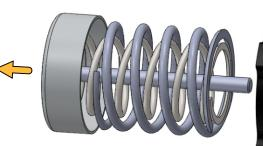
5. Install the new springs, ensuring they are correctly seated in the grooves at the bottom of the body, and on the underside of the piston
