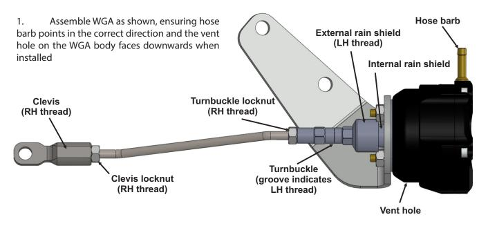
2. Ensure the clevis and turnbuckle have at least 5mm of thread engaged, but do not tighten any of the locknuts at this stage
