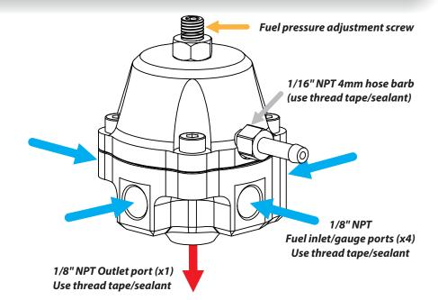
The FX-S has five fuel ports on the body (4 inlet/reference pressure, 1 outlet), all of which are 1/8" NPT. Please ONLY use NPT fittings, and note that whilst 1/8" BSP fittings look very similar and will seem to screw in, they will not provide a leak-proof joint.
