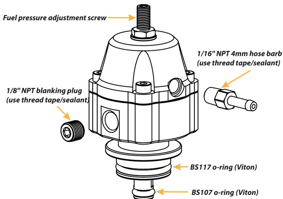
The FX-S has a single 1/8" NPT port on the body that can be used for a fuel pressure gauge/electronic pressure sensor, or it can be plugged with the supplied 1/8" NPT plug. Fuel-safe thread tape or sealant will be required on this thread to prevent a fuel leak. If using thread tape, ensure there is no tape on the leading edge of the thread as pieces of tape could break off and go into the fuel system.
