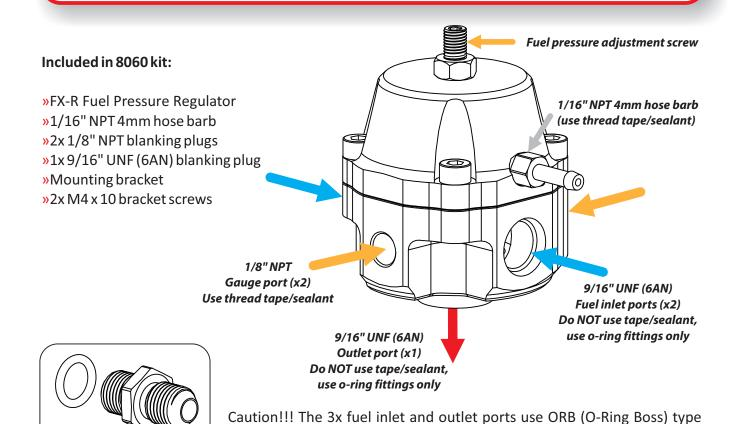
The remaining 2x ports on the FX-R body are 1/8" NPT and are intended to be used for either a fuel pressure gauge, an electronic fuel pressure sender, or both. If either of these outlets are not used, please block them with the provided 1/8" NPT pressure plugs. These WILL require a fuel-safe thread sealant.
