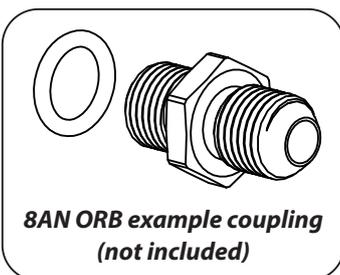
Caution!!! The 3x fuel inlet and outlet ports use ORB (O-Ring Boss) type fittings and adapters with a 3/4" UNF thread (8AN). Be aware that they are NOT pipe threads and do NOT use thread sealant - they are reliant on the o-rings for a positive seal. Please ensure that you use ORB-type fittings.
