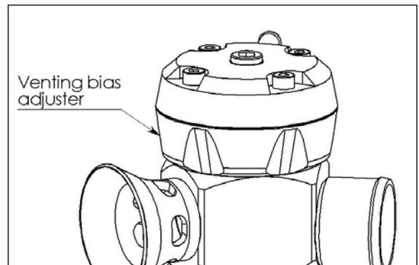
Typically, most engines will allow 100% atmosphere venting with no problems, provided the spring pre-load is adjusted correctly. However, some combinations of modifications can result in backfiring when the valve vents to atmosphere, in which case the solution is simply to dial back the amount of air vented to atmosphere until the problem is resolved – this is one of the key benefits of the venting bias adjustment feature.
