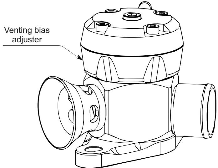
Typically, most un-modified engines will allow 100% atmosphere venting with no problems. However, some combinations of modifications can result in backfiring if high proportion of atmosphere venting is used, in which case the solution is simply to dial back the amount of air vented to atmosphere until the problem is resolved – this is one of the key benefits of the venting bias adjustment feature.
