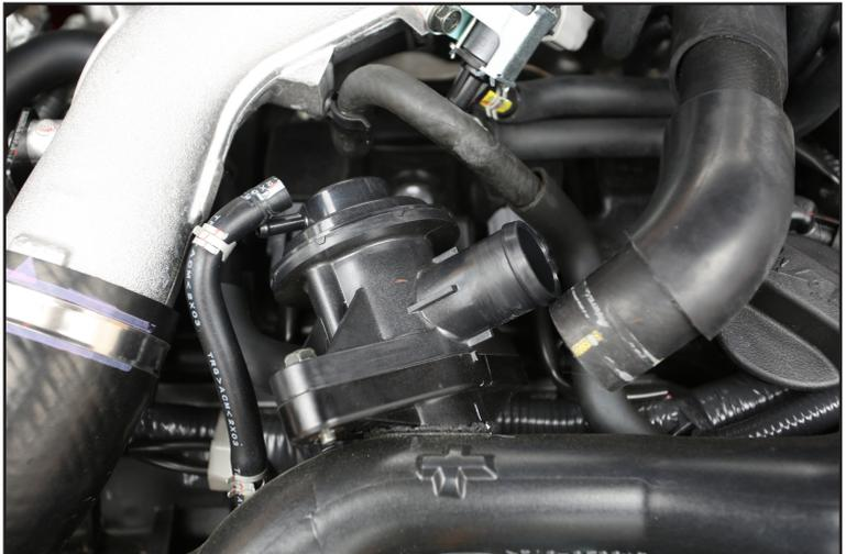
4) Fit the GFB valve to the intercooler, making sure the supplied red o-ring is fully inserted into the groove in the underside of the GFB valve as shown below.
