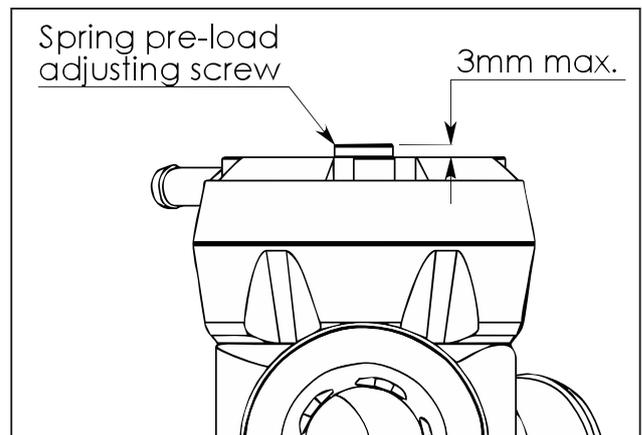
Take the car for a drive, and take note of how easily the valve vents when you lift off. Making the spring softer will allow the valve to open easier and vent longer, and increasing the pre-load means you will need to drive the car harder (i.e. more boost) before you start to hear the valve venting, and the blow-off sound will be shorter in duration.
