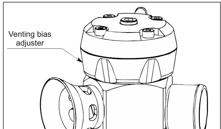
Do not be afraid to experiment with the spring and noise settings, as the air/fuel ratio cannot be affected regardless of the BOV settings, and it is not possible to damage the engine or turbo with BOV adjustments.
