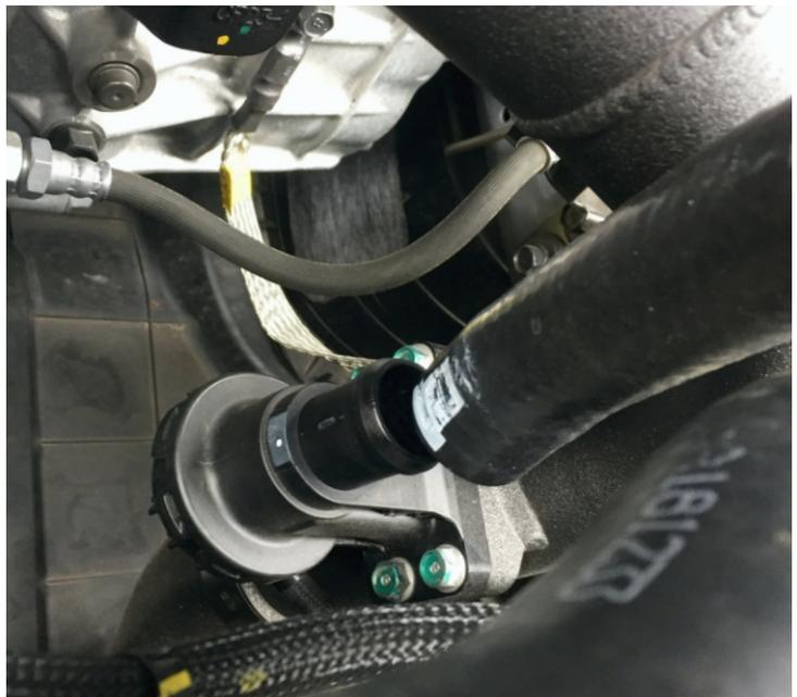
3) Ensure the brown o-ring is installed in the groove on the underside of the Respons valve, then install it back in the factory location using the supplied longer screws and 5mm hex key.
