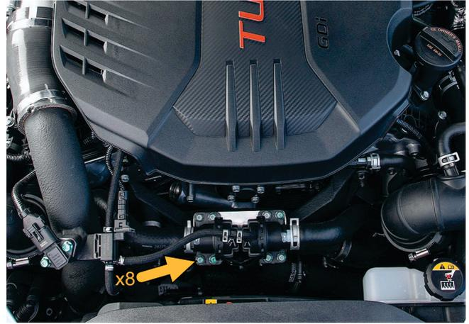
2) Ensure the brown o-rings are installed in the grooves on the underside of the GFB valves, then install them onto the engine using the supplied screws and 5mm hex key. The valves are oriented so the vacuum nipples point to the front of the car
