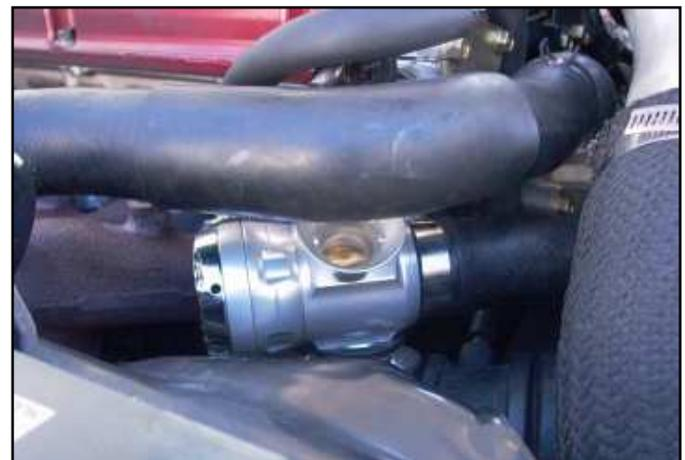
For custom hose mounting, a location for the Respons must be found on the piping between the turbo outlet and the throttle body, and a suitable adaptor must be welded in that location. A hose to connect the Respons recirc outlet must also be fitted to the piping before the turbo (after the airflow meter if one is installed).
