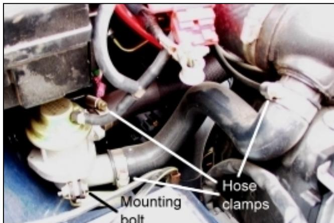
3) Remove the vacuum hose from the top of the factory valve (this hose is a tight fit, try using a flat screwdriver to push the hose off, rather than pulling it).
