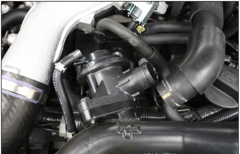
3) Remove the factory vacuum hose from the car, and replace it with the longer piece supplied in the kit. Hose clamps or cable ties are not required on this hose
