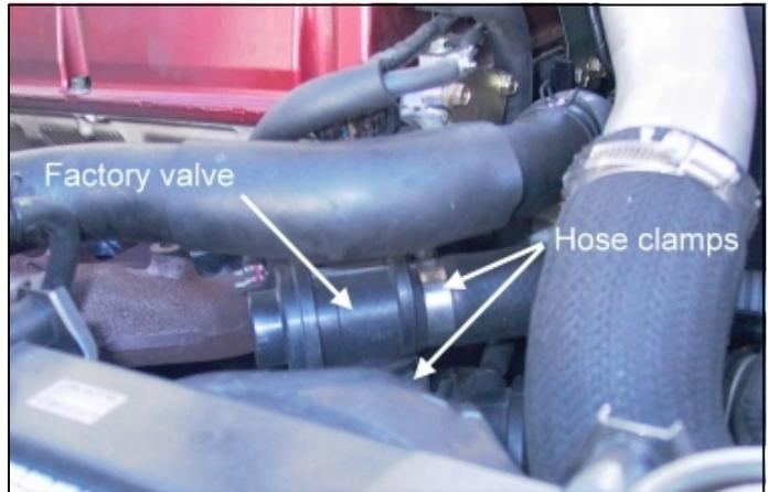
For custom installations or cars without a factory fitted valve, a location for the Mach 2 must be found on the piping between the turbo outlet and the throttle body, and a suitable adaptor must be welded in that location to which a 1.25" hose can be connected.
