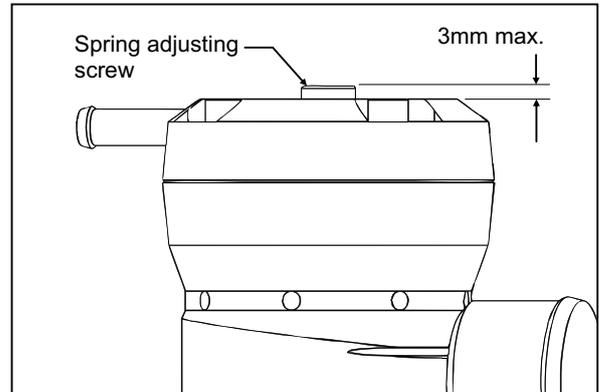
It is possible to use the Mach 2 straight out of the box without any spring pre-load adjustments, however you can use the adjustment to fine-tune throttle response. Generally speaking, the hardest spring pre-load you can run without causing compressor surge (fluttering sound when lifting off the throttle) is ideal.
