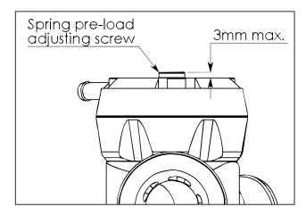
the spring softer will allow the valve to open easier and vent longer, and increasing the pre-load means you will need to drive the car harder (i.e. more boost) before you start to hear the valve venting, and the blow-off sound will be shorter in duration.
