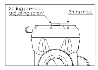
spring softer will allow the valve to open easier and vent longer, and increasing the pre-load means you will need to drive the car harder (i.e. more boost) before you start to hear the valve venting, and the blow-off sound will be shorter in duration.
