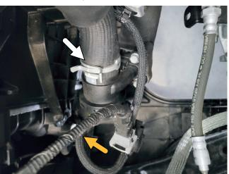
4) Loosen the top clamp () on the metal intercooler pipe, then pull it free of the hose:
