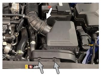
2) Remove the two plastic clips on the intake, followed by the 3 bolts that hold the lower half of the airbox ( ). Carefully remove it from the car and set aside:
