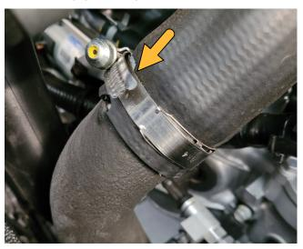
5) Bend the top of the pipe towards the engine ( ) to allow access to remove the four screws on the factory diverter valve ( ):
