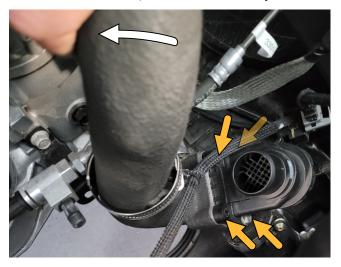
6) Install the GFB valve using the supplied screws. A 5mm T-handle hex key helps with the rear screws:
