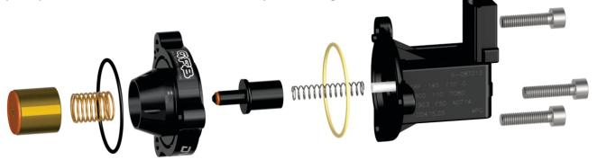
**Please note:** the amount of force required to "snap" the DV+ body onto the solenoid varies because the solenoid is moulded plastic - some solenoids are quite loose and need to be held together until it is bolted onto the car, others can be quite tight and need a good deal of force (by hand). This variation in factory moulding tolerance does not affect the operation in any way.
