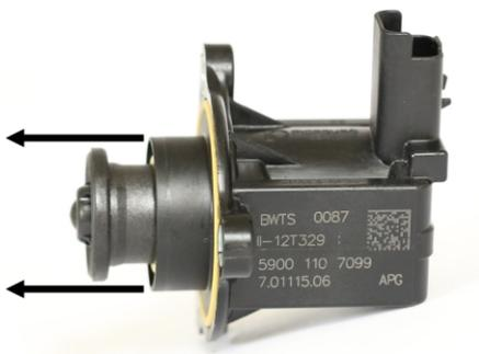
Pull on the plastic diaphragm shroud, the whole assembly will pop off leaving the bare solenoid coil. Keep the yellow o-ring.
