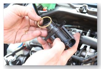
2. Using a flat screwdriver in the o-ring groove, carefully pry the piston surround from the solenoid body.
