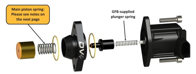
Note that the bolt holes are NOT SYMMETRICAL. When you assemble the DV+ body onto the solenoid body, check the alignment of the holes - if they do not line up properly, rotate the DV+ body 180 degrees and check that they line up correctly before installing on the car.
