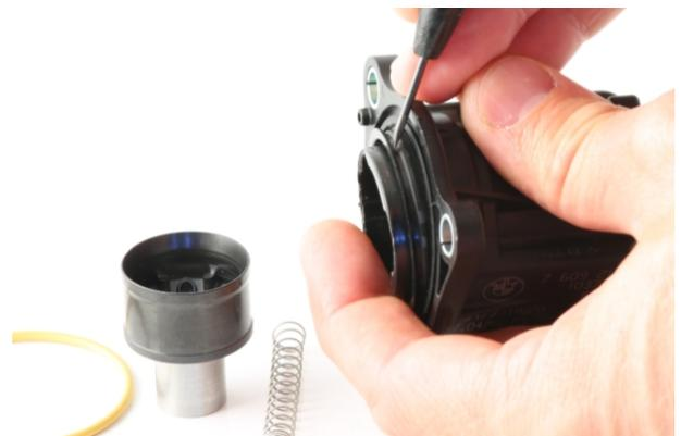
Assemble the GFB parts onto the factory solenoid body as shown in the exploded view below, making sure to use the GFB-supplied plunger spring, and the yellow o-ring removed from the factory valve. Apply some engine oil to the piston during this process.
