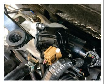
On Renault Clio RS engines, the factory diverter is mounted on a plastic housing joined by hoses. There is also a mounting bracket that holds the housing in place. It is easiest to first remove the screws holding this housing, which makes it easier to access the three screws that retain the factory diverter.
