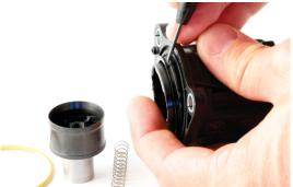
Pull the piston and spring out of the body, then remove the yellow o-ring. This will leave the plastic ring indicated by the arrow, which MUST BE REMOVED before the DV+ is installed. Lever it gently and work your way around.
