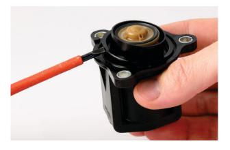
Assemble the GFB parts onto the factory solenoid body as shown in the exploded view below, making sure to use the GFB-supplied plunger spring, and the yellow o-ring removed from the factory valve. Apply some engine oil to the piston during this process, and check that the piston moves freely.
