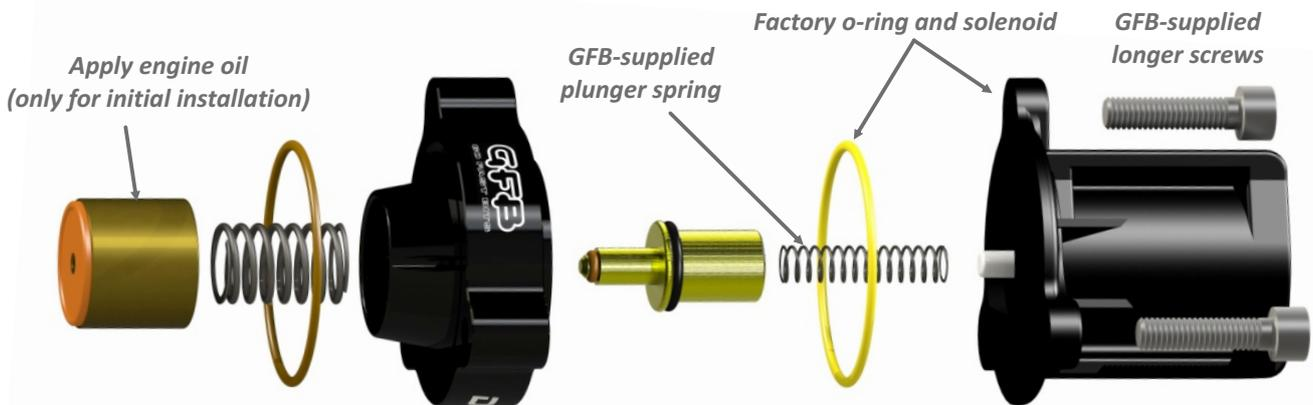
During assembly, check that the piston slides freely in the body without sticking or binding. It is a very close fit and can sometimes be difficult to get started into the bore, but once in it should move without needing to be forced. Apply some engine oil onto the piston during assembly. **It is NOT necessary to regularly lubricate the piston after assembly.**
