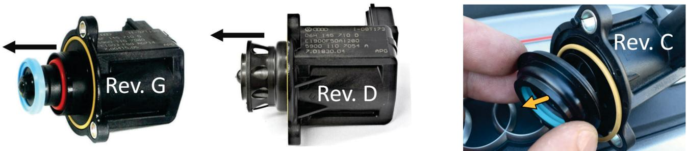
Pull on the diaphragm shroud (revision G), or the plastic “basket” (revision D), and the whole assembly will pop off leaving the bare solenoid coil. For revision C, first pull the piston from the body and remove the spring. Then remove the piston shroud - this can usually be pulled out by hand, but if it's too tight, it can be carefully levered out with a flat screwdriver. The thin plastic may be damaged, however it is not re-used in the VTA installation.
