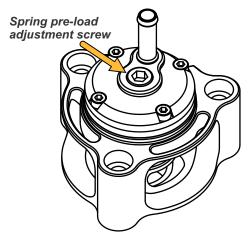
Adjusting the spring pre-load changes how easily the valve vents when the ECU triggers. The best throttle response is typically found when the spring is set as firm as possible without causing compressor surge (turbo fluttering) when the throttle is closed on a high boost/high RPM gearshift.
