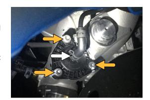
Before installing the VTA, check that the sealing orings are installed in the grooves on the VTA body as shown opposite.
