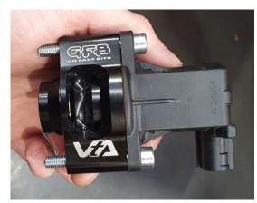
Note that the bolt holes are NOT SYMMETRICAL. When you assemble the VTA onto the solenoid, check the alignment of the holes - if they do not line up properly, rotate the VTA body until the bolt holes line up correctly before continuing.
