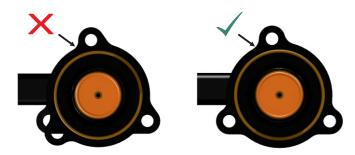
Install the VTA assembly onto the turbo using the supplied longer screws. Because of the asymmetric bolt holes, the assembly can only be installed in one orientation.
