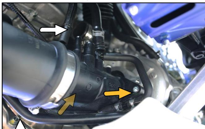
3) Using a 10mm socket, remove the two bolts that hold the turbo intake pipe onto the turbo.
