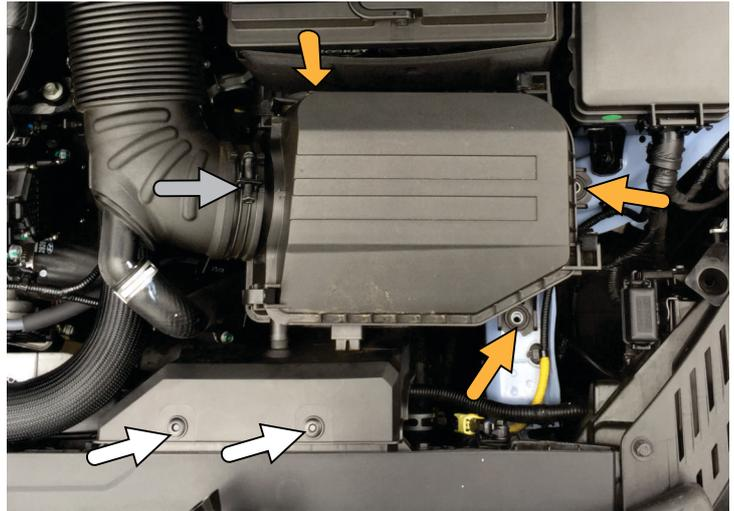
2) Before unbolting the factory valve, it is easiest to first remove the recirc hose while the valve is still solidly mounted (this hose is quite tight and needs some wiggling persuasion). Then remove the factory valve from the car using a 10mm socket for the 4 screws.
