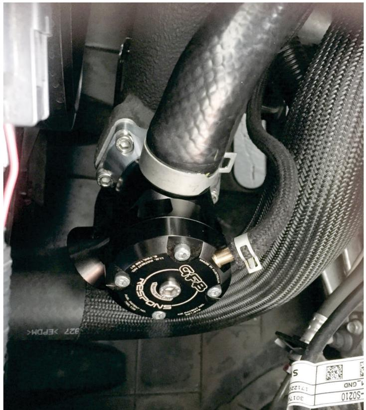
6) Fit the recirc and vacuum hoses onto the Deceptor Pro II, and replace the clamps.
