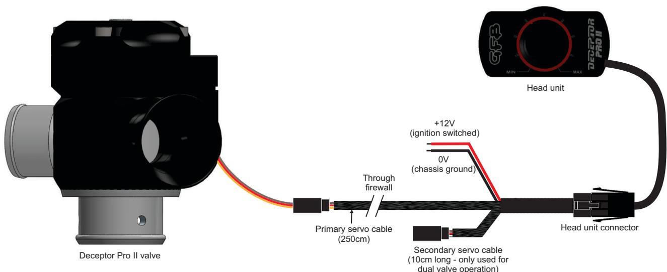
Feed the primary servo cable through the firewall into the engine bay. Ensure that the cable is protected where it passes through the firewall to prevent shorting out.
