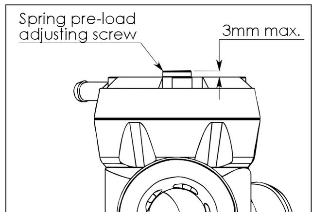
Take the car for a drive, and note how easily the valve vents when you lift off. Making the spring softer will allow the valve to open easier and vent longer, and increasing the pre-load means you will need to drive the car harder (i.e. more boost) before you start to hear the valve venting, and the blow-off sound will be shorter in duration.
