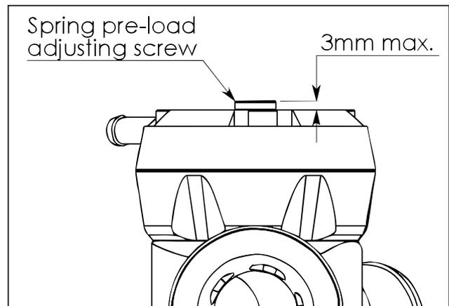
Take the car for a drive, and take note of how easily the valves vent when you lift off. Making the springs softer will allow the valves to open easier and vent longer, and increasing the pre-load means you will need to drive the car harder (i.e. more boost) before you start to hear the BOVs venting, and the blow-off sound will be shorter in duration.
