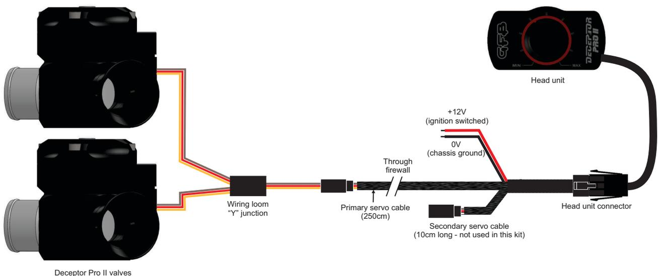
Continue the installation by feeding the primary servo cable through the firewall into the engine bay. Ensure that the cable is protected where it passes through the firewall to prevent shorting out.
